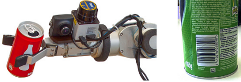
Fig. 6. The eye-in-hand camera mounted on the manipulator (left) and a typical image captured by this camera during object inspection (right).
