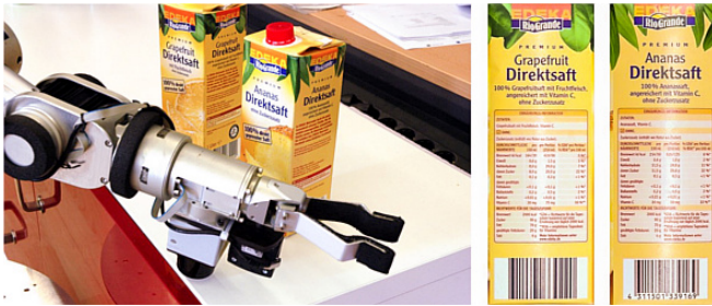
Fig. 9. The eye-in-hand camera positioned to capture the text label of a pineapple juice/"Ananas" (right object). It is of similar appearance as grapefruit juice (left object). They differ in their barcode and text labels naming their flavours. Texture is very similar. They are of the same color.
