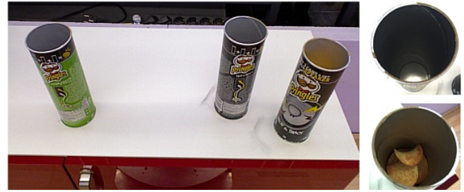
Fig. 10. Input image for initial recognition (left) of the scene and inspection images during inspection of the property "fill level" (right). Objects from left to right: onion chips, an empty and a full "hot and spicy" chips can.
