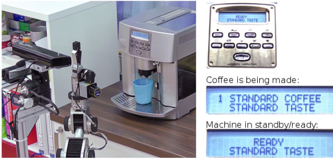
Fig. 8. The robot getting the property (mode of coffee machine) by reading the display of the coffee machine (left). The control panel and two messages on the display telling that one coffee is being made and the machine being in standby/ready (right).
