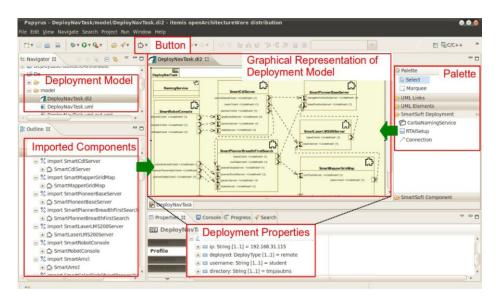
Figure 6: SmartSoft MDSD Toolchain reusing components
