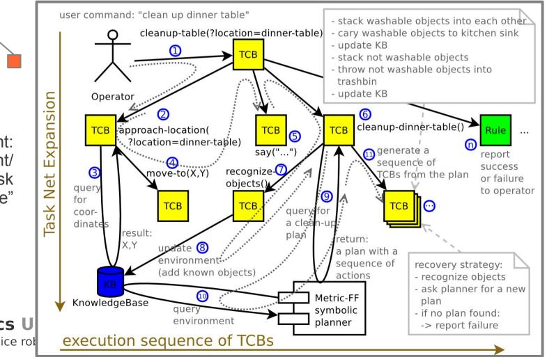
On the right: example for a refinement/ expansion of the task "cleanup-table"
