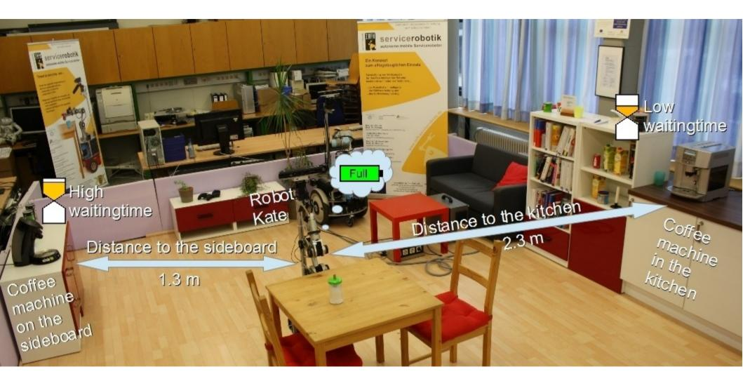
The robot needs to trade-off different non-functional properties such as **safety** and **performance** in order to select appropriate execution variants (in this case which coffee machine to use)
